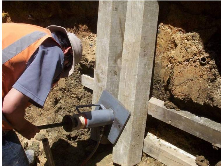
**Figure 6: In-situ shear strain verification test**
