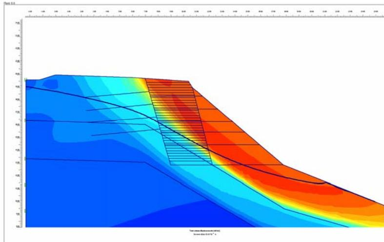
**Figure 2:** Typical Design Cross-Section showing proposed solution superimposed on failed surface
