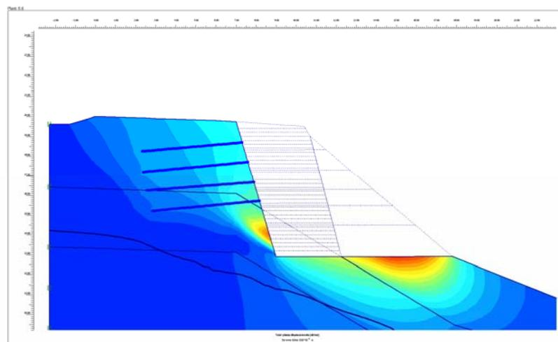
**Figure 7: Temporary excavation deformation check (est. 8mm)**
