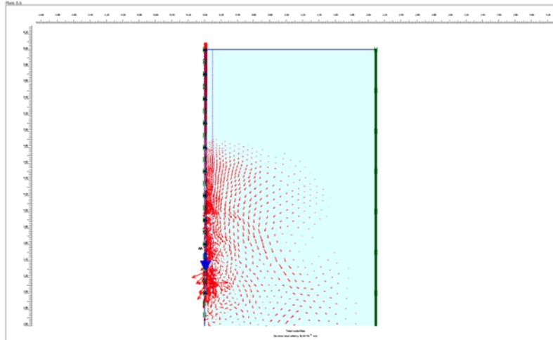
**Figure 4:** Output showing predicted phase velocity\* during installation of nail.
