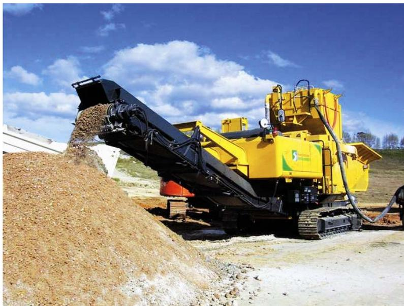
**Fig 3. Reterra mobile soil recycler in use at the NZ Navy Whangaparaoa firing range site. (Case study 5) (photo Hiway Stabilizers Environmental Ltd 2004)**
