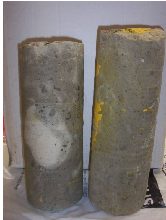
Figure 12: Sample cores Mix Design 2 (Homogenous Columns with 6% lime )
