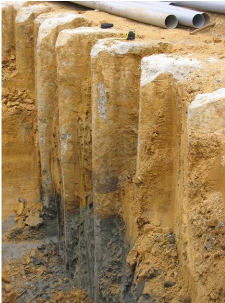
Figures 9 & 10: Photos showing exposed trial columns
